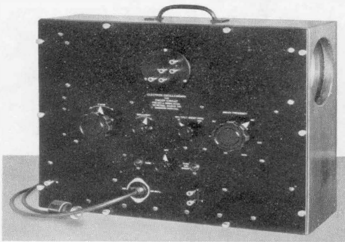
The new Electron Oscillograph (TYPE 687-A) includes sweep circuit and power supply
